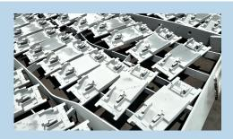
ASSEMBLY AND PACKING ZINGANIZED BASEPLATES ARE DRIED TO PERFECTION AND ARE THEN ASSEMBLED AND PACKED FOR THE CLIENT – READY FOR USE ZINGANIZATION BASEPLATES ARE ZINGANIZED USING AN AIRLESS SPRAY GUN. TWO COATS OF 60µ OF ZINGA IS APPLIED ONTO THE SURFACE. (120µ IN TOTAL)
