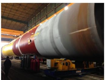
In 2014 ZINGA was used on the construction of new wind mills for Dutch energy provider ENECO. ZINGA was chosen to protect the most sensitive parts of the windmills: the monopile's external primary steel, +3m of mudline to -2m below of mudline. Also the top of the monopile flange was treated with ZINGA (2 x 90  $\mu$ m DFT).
