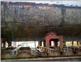
In February 2013, a Navy ship was treated with ZINGA in duplex with the LioCyl fouling release system in a black colour.
