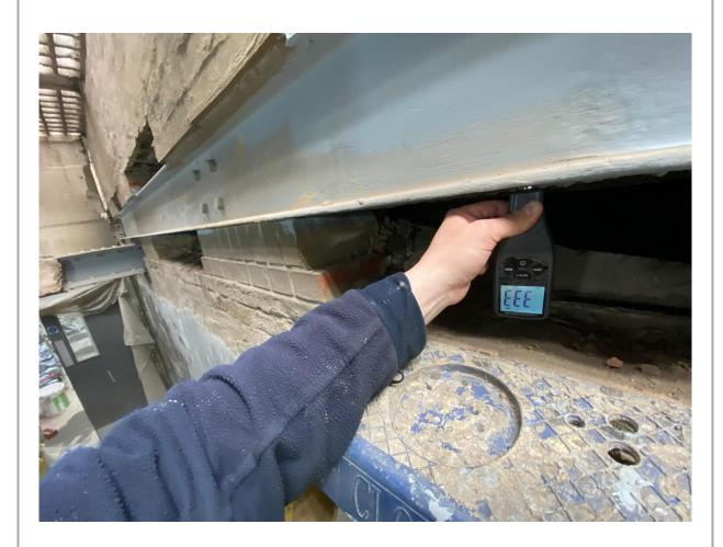
1. This reading shows 333 $\mu$ m DFT, and this is excessive. Where 180  $\mu$ m DFT has been specified, we work to SSPC-PA2 like thousands of other people in the industry, and the upper threshold limit that we work to is always 120% of the specified figure. In this case it is 180 x 120% = 216 (220 rounded-up). This beam looks like a new installation, so without seeing the 'before' photos it looks very high.
