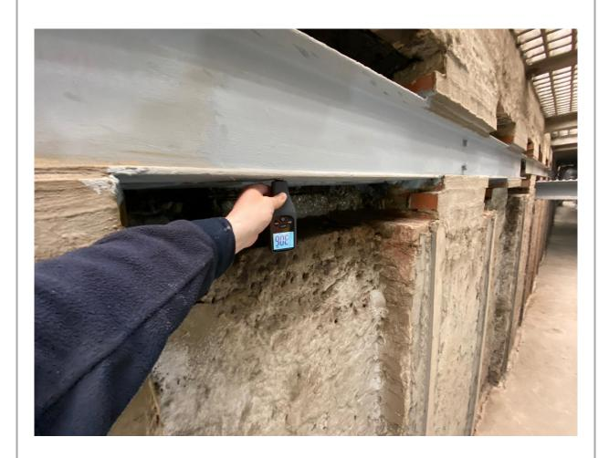
3. This reading is showing a value of  $306\mu m$  DFT and the beam looks like a new one, so without any 'before' photographs we have to assume that the reading is very high. If it is a new beam with hih readings, then the coating must be checked carefully for micro-cracking on inside corners where the film-build tends to be higher.
