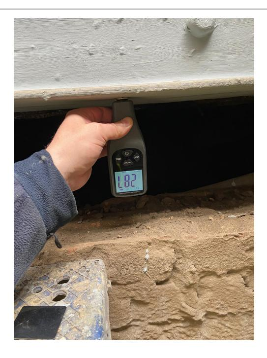
2. This fgure of  $287\mu m$  DFT could be a very high reading, or there could be surface undulations or 'scalloping' over a small area. This is the reason that coating inspectors take spot-readings ie three readings taken within the size of a hand. If two are showing, for example, 220 and one is showing 300  $\mu m$  DFT then the chances are that it is an errneous reading.
