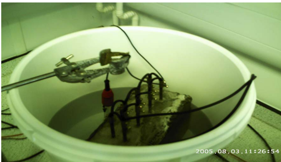
Figure 21 Concrete block one experimental set up
