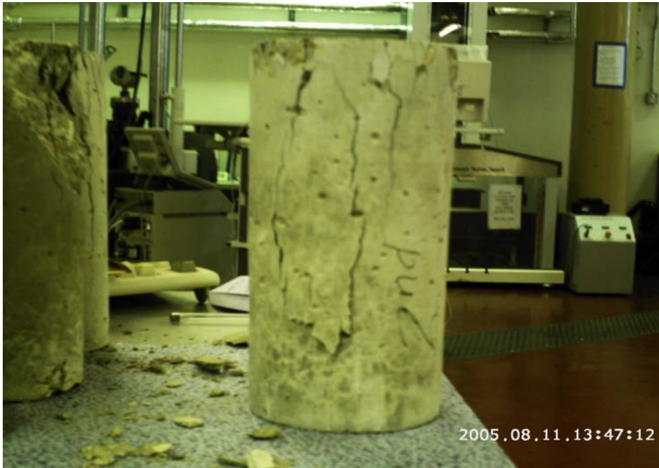
Figure 25 Concrete cylinder one after compression test
