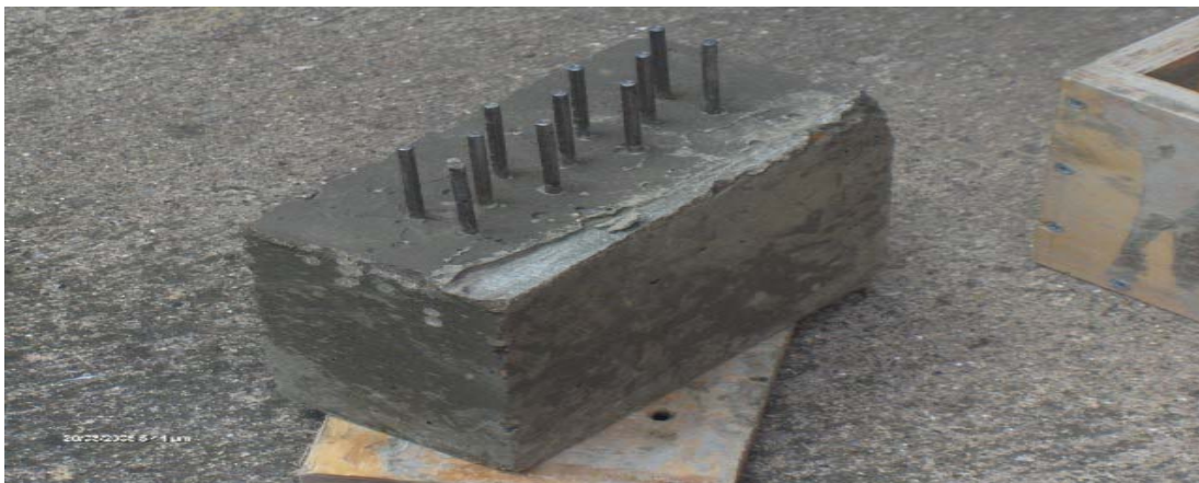
Figure 13 Concrete sample removed from the mould.
