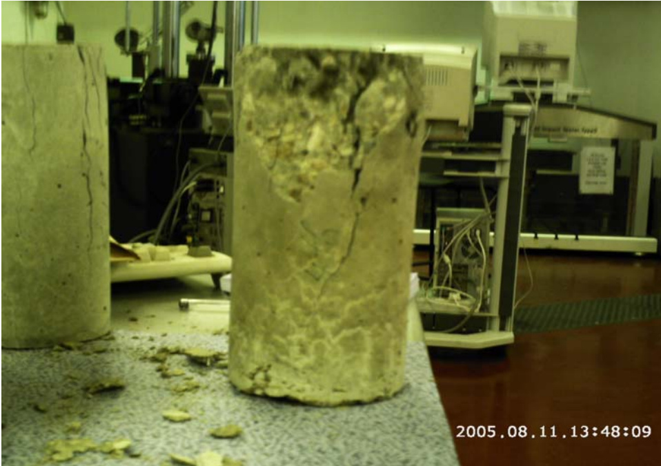
Figure 27 Concrete cylinder three after compression test
