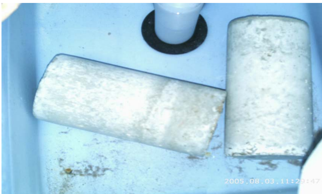
Figure 17 Cylindrical Concrete curing in fresh water bath.
