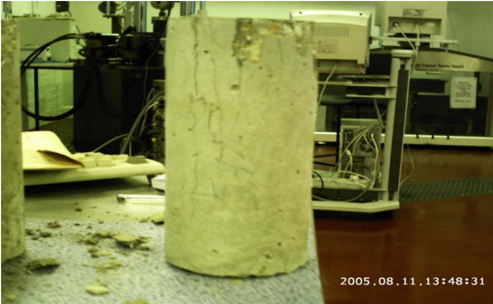
Figure 28 Concrete cylinder four after compression test.
