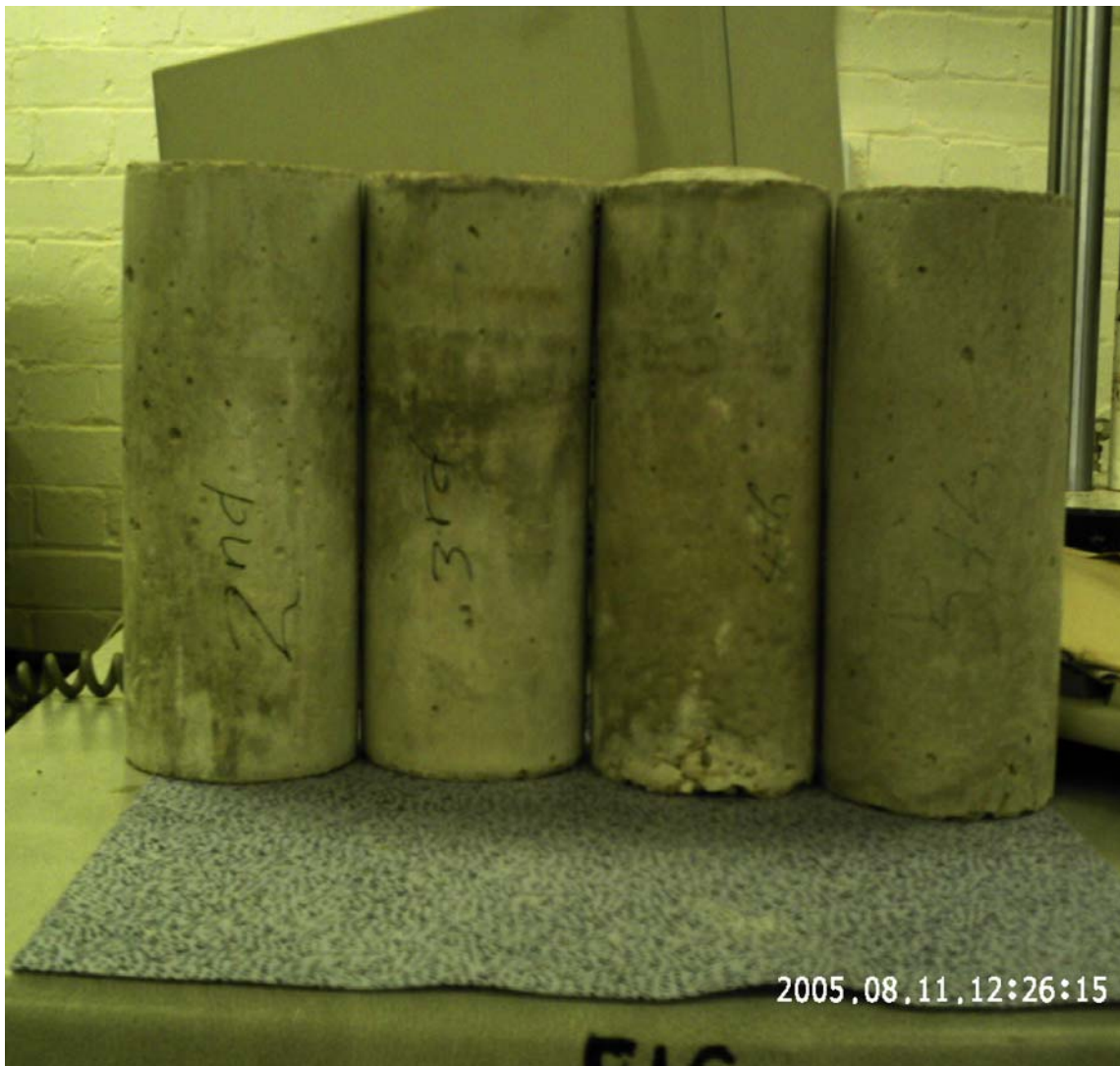
Figure 24 The four concrete cylinders before compression test.
