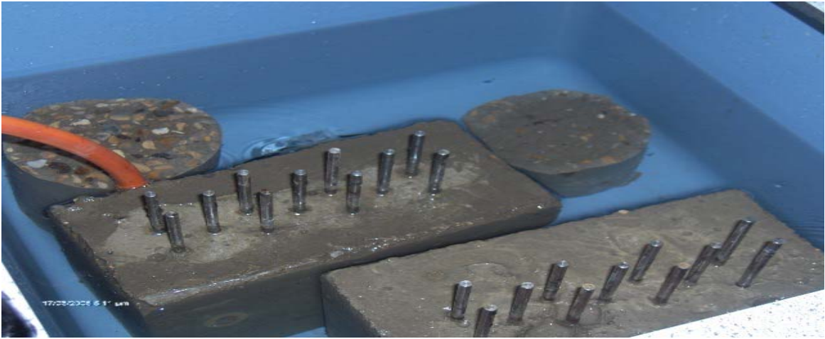
Figure 14 Concrete samples in fresh water during curing
