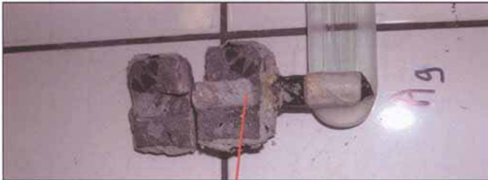
Thin layer of cement and Zinga on steel rod
