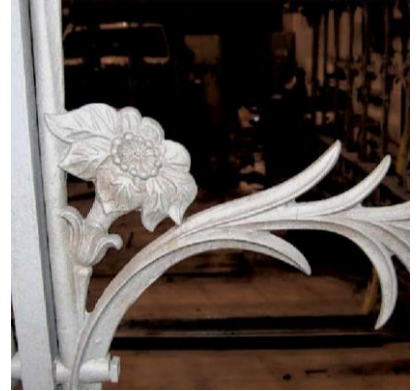
Etching by means of micro glass flakes
