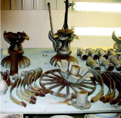
Etching the surface has allowed to determine the deterioration of certain elements.
