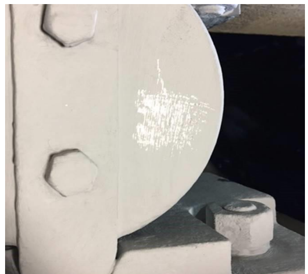
After application of ZINGA . The picture on the right shows shiny metallic zinc after a coin rub test was performed.
